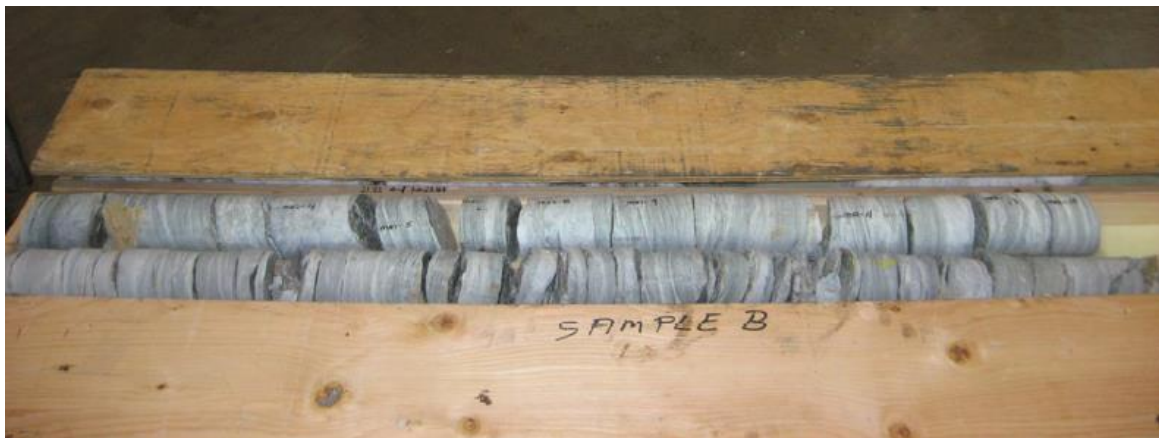
Figure 13-4 : Platey Breakage Example on Core Sample B
